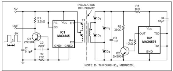
Figure 1. This temperature sensor (IC2, the MAX6576) is isolated by the transformer, and provides a digital output whose period encodes the temperature (10μs/°K to 640μs/°K).
