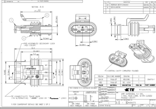
3 pos AMP Superseal 1.5 with closed cavities - drawing proposed
