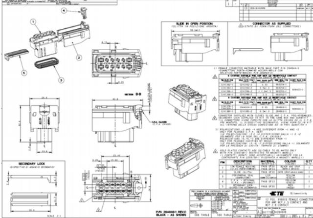
12 pos MCP sealed female connector - drawing proposed
