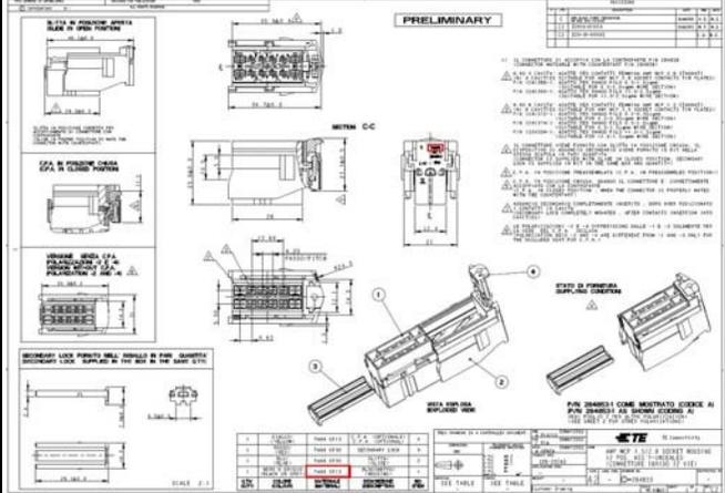
12 pos MCP sealed female connector - drawing in force
