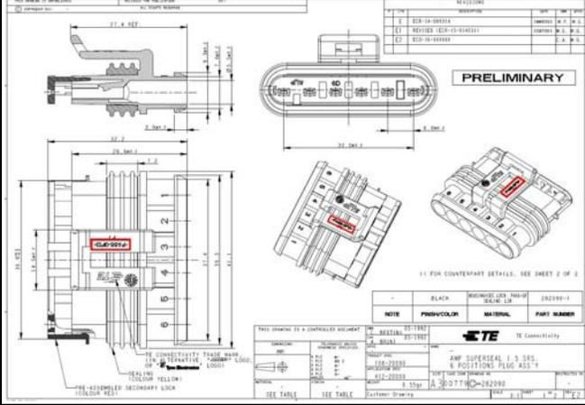
3 pos AMP Superseal 1.5 with closed cavities - drawing in force
