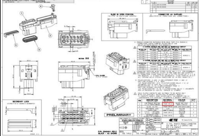
20 pos MCP unsealed female connector - drawing in force
