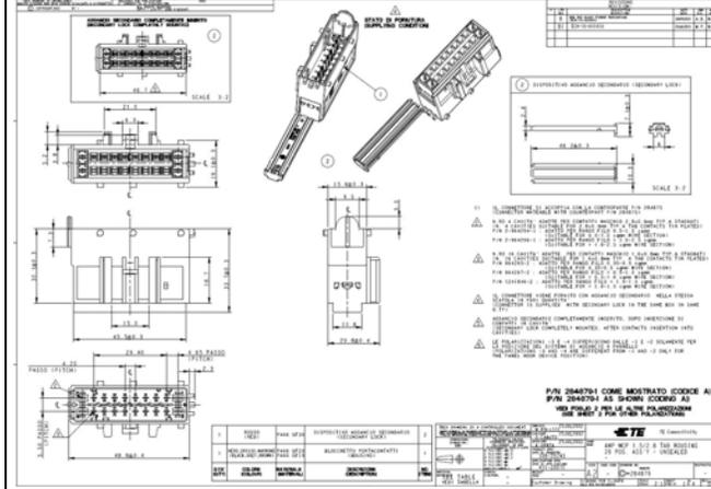
20 pos MCP unsealed male connector - drawing proposed
