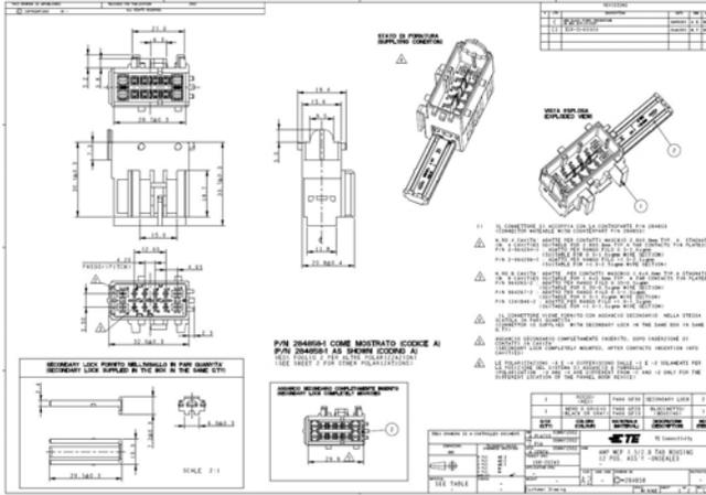
12 pos MCP unsealed male connector - drawing proposed
