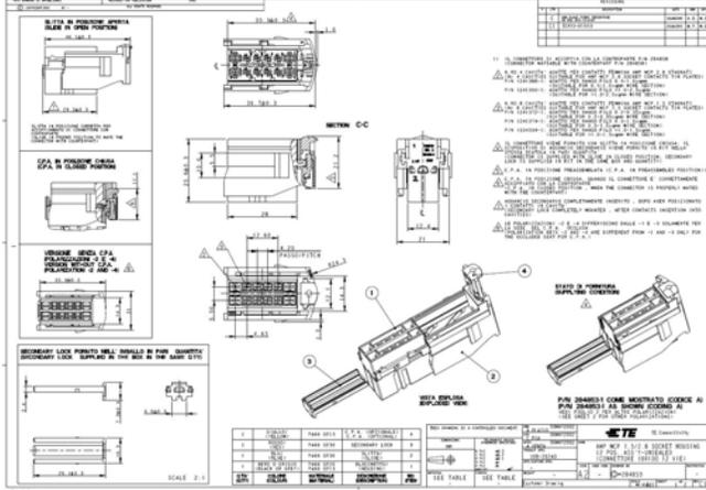
12 pos MCP unsealed female connector - drawing proposed
