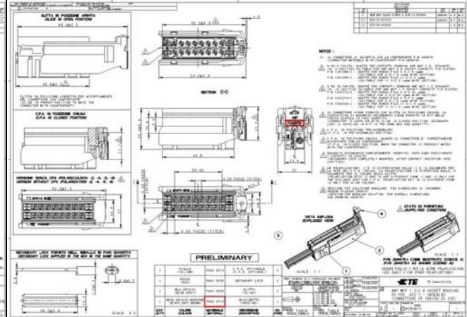
20 pos MCP unsealed male connector - drawing in force
