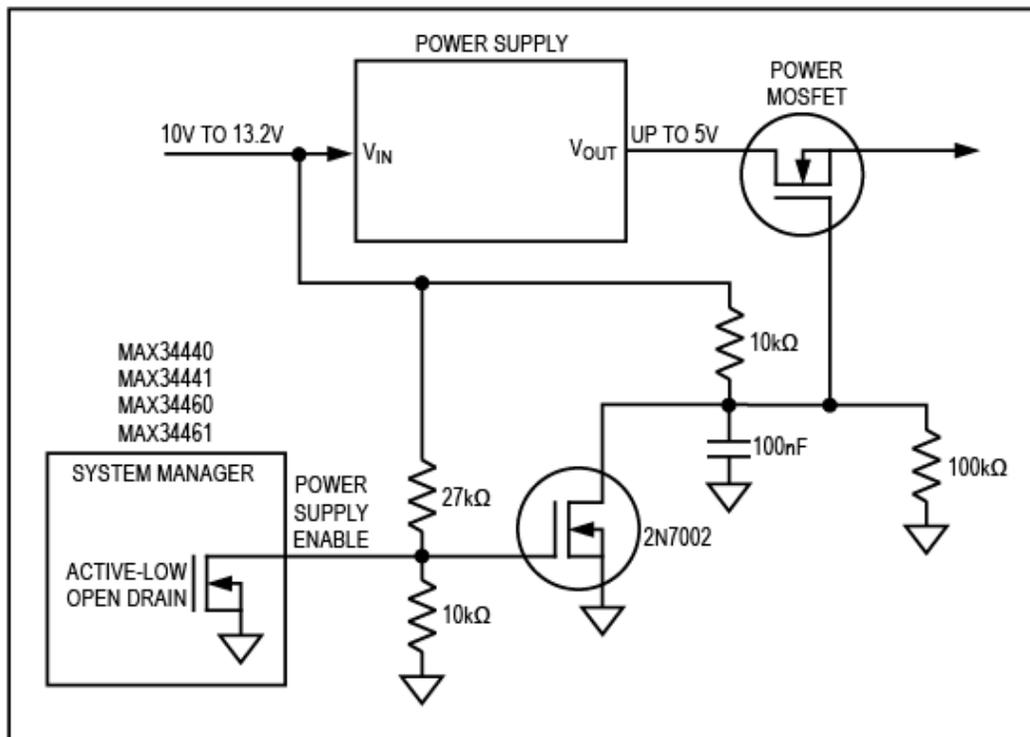
Figure 1. Level-shifting circuitry.
