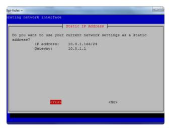
The installer will automatically try to set the dynamic IP address it got from your router to be fixed. This works well enough, if you have an advanced network set up, you can configure a custom IP address
