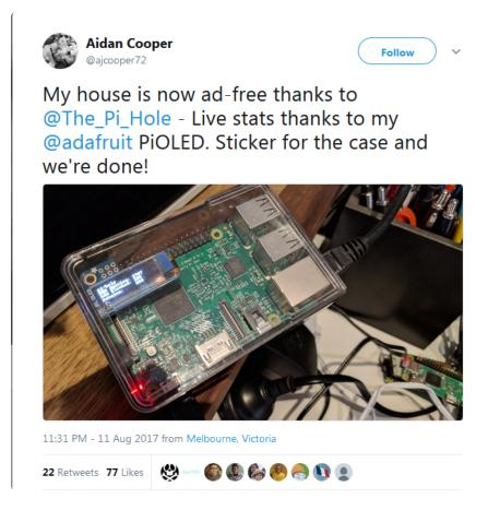
What a perfect use! Here's how to add it on for some nice stats. It also displays the hostname and IP address so if you forget it you can just look at the display. It will also tick up when its in use so you can tell its working.
