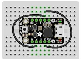
This wiring example shows A1 and A2 connected to ground.
