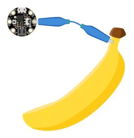
You may need to reload your code or restart your board after changing the attached item because the capacitive touch code "calibrates" based on what it sees when it first starts up. So if you get too many touch responses or not enough, reload your code through the serial console or eject the board and tap the reset button!
