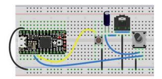
Wiring is the same for the M4 versions of the boards as it is for the M0 versions. Follow the same image for both.
