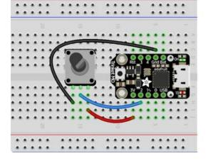
A1 is labeled as 2! It's located between "1" and "3V" on the same side of the board as the little red LED. Ground is located on the opposite side of the board. 3V is located next to 2, on the same end of the board as the reset button.
