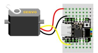
For QT Py M0, connect the ground wire to GND, the power wire to 5V, and the signal wire to A2.
