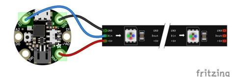
Note that the wire ordering on your NeoPixel strip or shape may not exactly match the diagram above. Check the markings to verify which pin is DIN, 5V and GND
