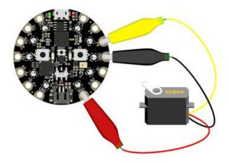
For Circuit Playground Express and Circuit Playground Bluefruit, use jumper wire alligator clips to connect the ground wire to GND, the power wire to VOUT, and the signal wire to A2.
