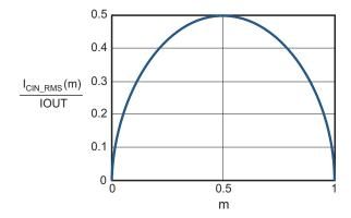
Figure 2. I<sub>CIN</sub> vs. Voltage Conversion Ratio
