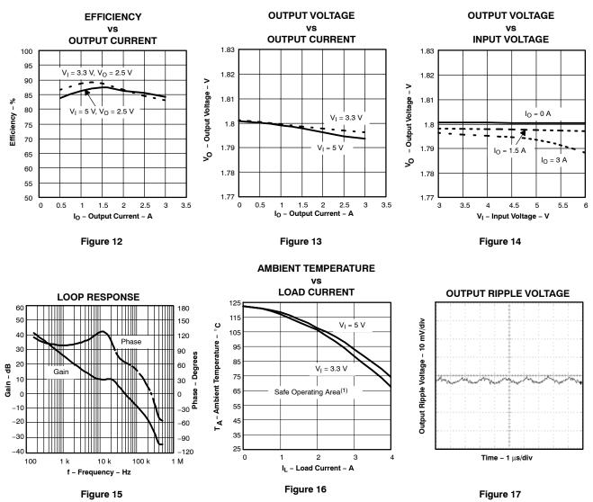
(1) Safe operating area is applicable to the test board conditions in the Dissipation Ratings
