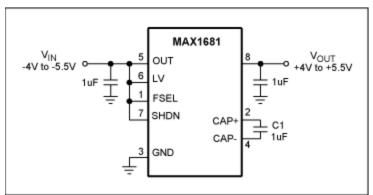
Figure 1. This switched-capacitor converter converts -5V to +5V.
