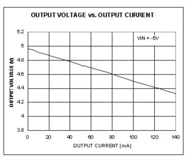
Figure 2. In Figure 1, the converter's non-zero output impedance results in an output voltage less than the ideal +5V.
