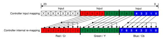
Figure 7-4. RGB-565 and YCbCr-565 I/O Mapping
