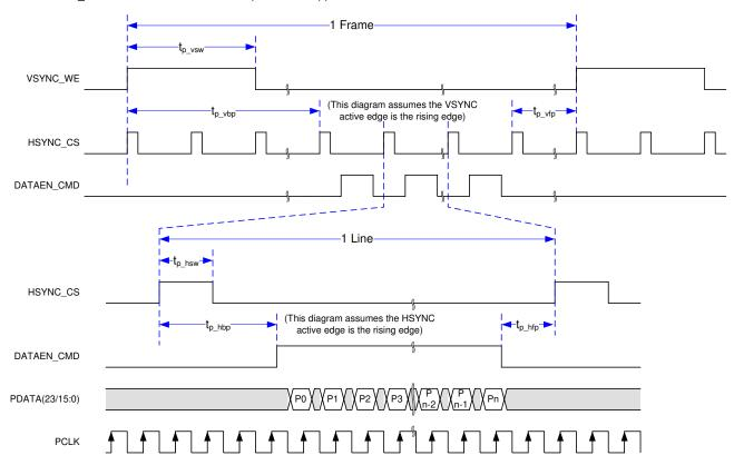
Figure 6-7. Parallel Interface Frame Timing
