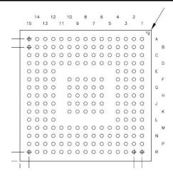
Figure 5-2. ZEZ Package 201-Pin NFBGA Bottom View
