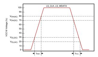
Figure 6-4. LS\_CLK and LS\_WDATA Slew Rate
