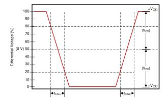
$V_{\text{CM}}$  is removed when the signals are viewed differentially.
