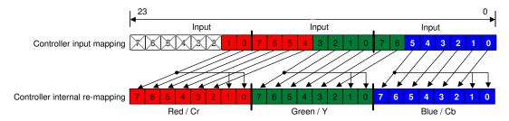
Figure 7-3. RGB-666 and YCbCr-666 I/O Mapping
