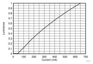
Figure 8-3. Typical Luminance vs Current
