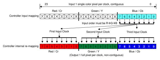
Figure 7-6. 8-Bit RGB-888 or YCbCr-888 I/O Mapping
