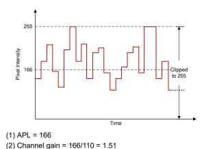
Figure 7-10. Source Pixels for a Color Channel
