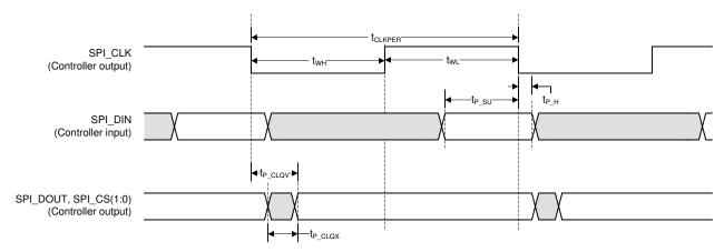
Figure 6-10. Flash Interface Timing
