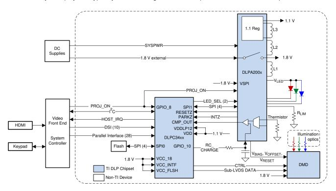
Figure 8-1. Typical Application Diagram (using DLPA200x)
