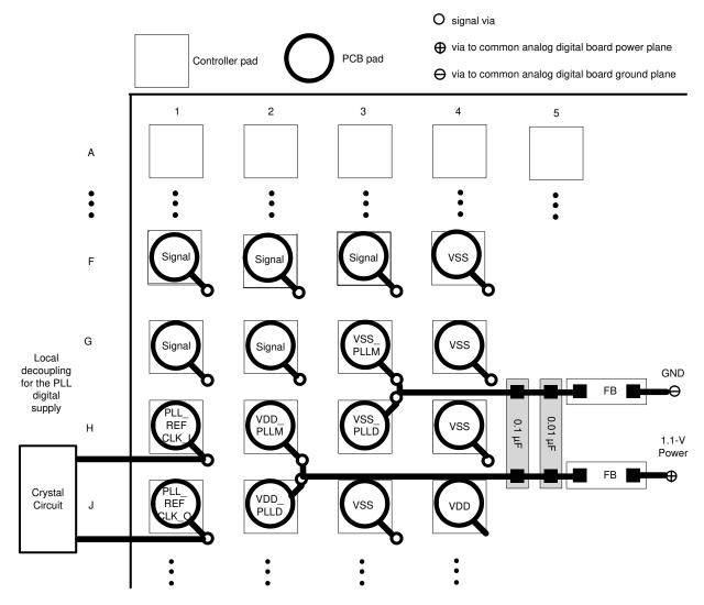
Figure 10-1. PLL Filter Layout
