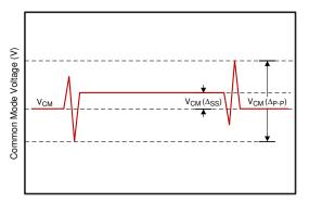
Figure 6-1. Common Mode Voltage
