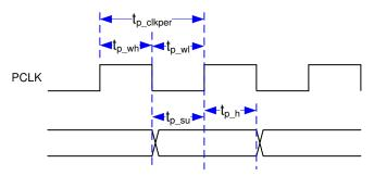
Figure 6-8. Parallel Interface Pixel Timing
