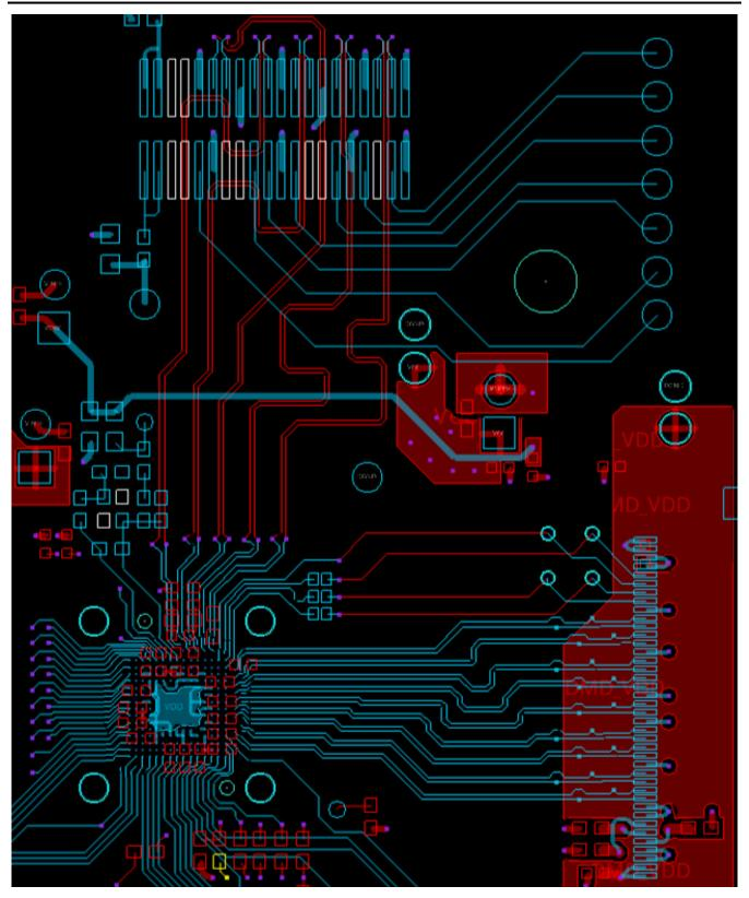
Figure 10-4. Layout Recommendation with DSI (DLPC3433 only)
