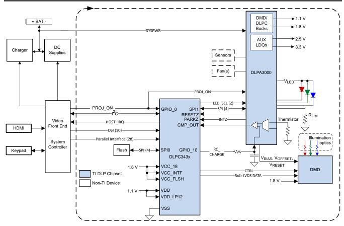
Figure 8-2. Typical Application Diagram (using DLPA3000)
