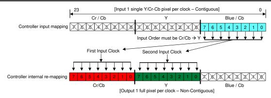
Figure 7-7. 8-Bit Serial YCbCr-422 I/O Mapping
