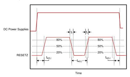
Figure 6-6. Power-Up and Power-Down RESETZ Timing
