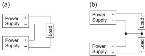
Fig. 4.1 Examples of series operation
