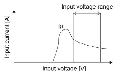
Fig.2.2 Input current characteristics
