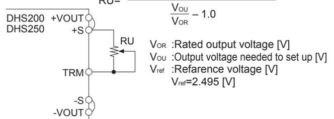
Fig. 3.8 Connection for output voltage increasing (DHS200/250)
