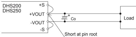
Fig. 3.2 When Remote Sensing is Not Used (DHS200/250)
