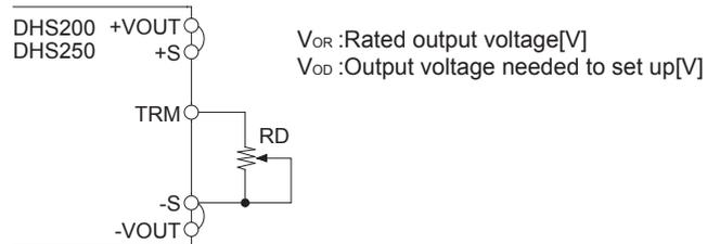
Fig. 3.7 Connection for output voltage decreasing (DHS200/250)
