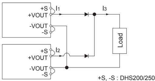
Fig. 4.2 Example of Redundancy Operation
