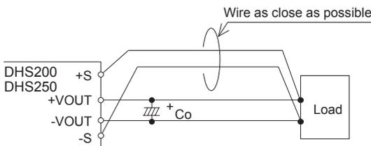
Fig. 3.3 When Remote Sensing is Used (DHS200/250)
