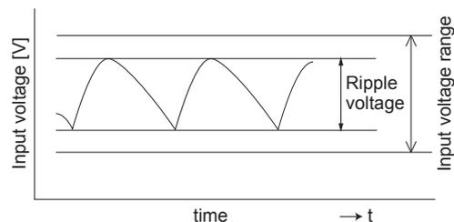
Fig.2.1 Input voltage ripple
