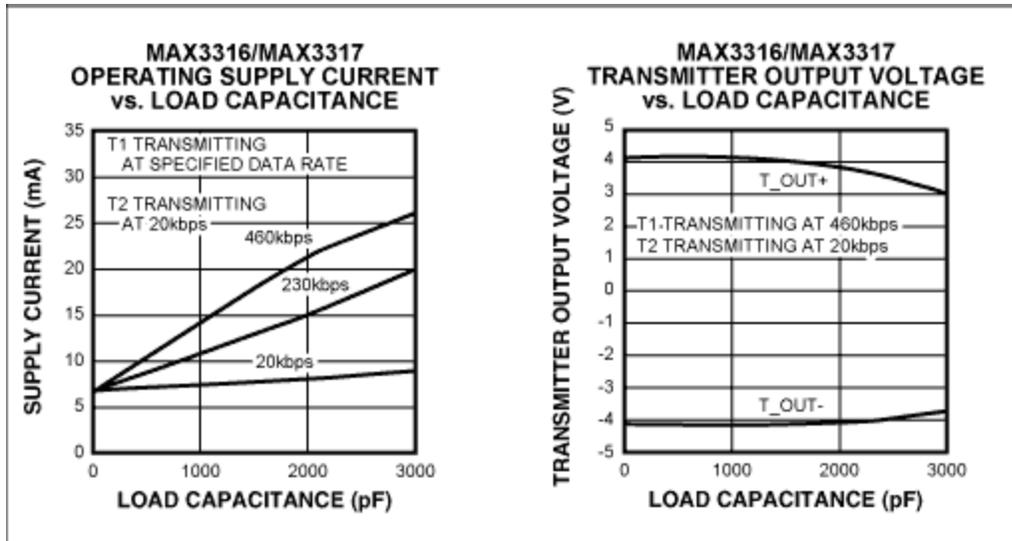
Figure 3. The MAX3316E draws low supply current from a 2.5V supply (left). Its transmitter-output voltages (right) are compatible with the RS-232 specification and compliant with the EIA/TIA-562 specification.
