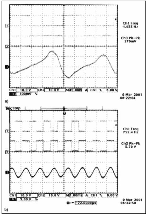
Figure 2. These Figure 1 waveforms, produced by two targets 180° apart, illustrate low- and mediumspeed operation: 4.9Hz at 2.4 revolutions/sec (a), and 752.4Hz at 376.2 revolutions/sec (b). Channel 1 is VOUT, Channel 2 is Acitve-Low VOUT, and Channel 3 is the voltage across R1.
