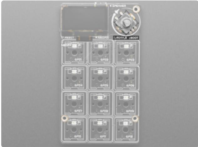
On the top right corner of the board (when viewed from the top), is the rotary encoder / BOOT button. The rotary encoder has 20 detents per rotation. The BOOT button is required to enter the bootloader (needed for both CircuitPython and Arduino), and is also available as a user input in code. To use the button, simply press the rotary encoder down.
