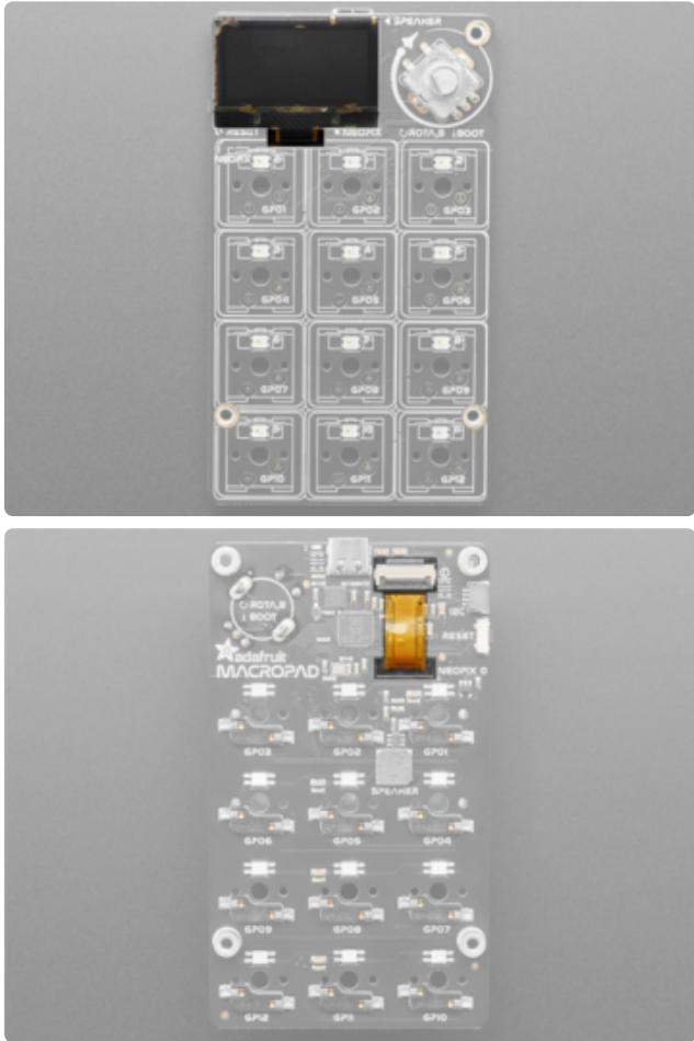
On the top left corner of the board (when viewed from the top), is the 128x64 SH1106 Monochrome OLED display. The ribbon cable for the display goes through a hole in the board to the back, where it is inserted into the display connector. This OLED is on high-speed hardware SPI to ensure quick updates.
