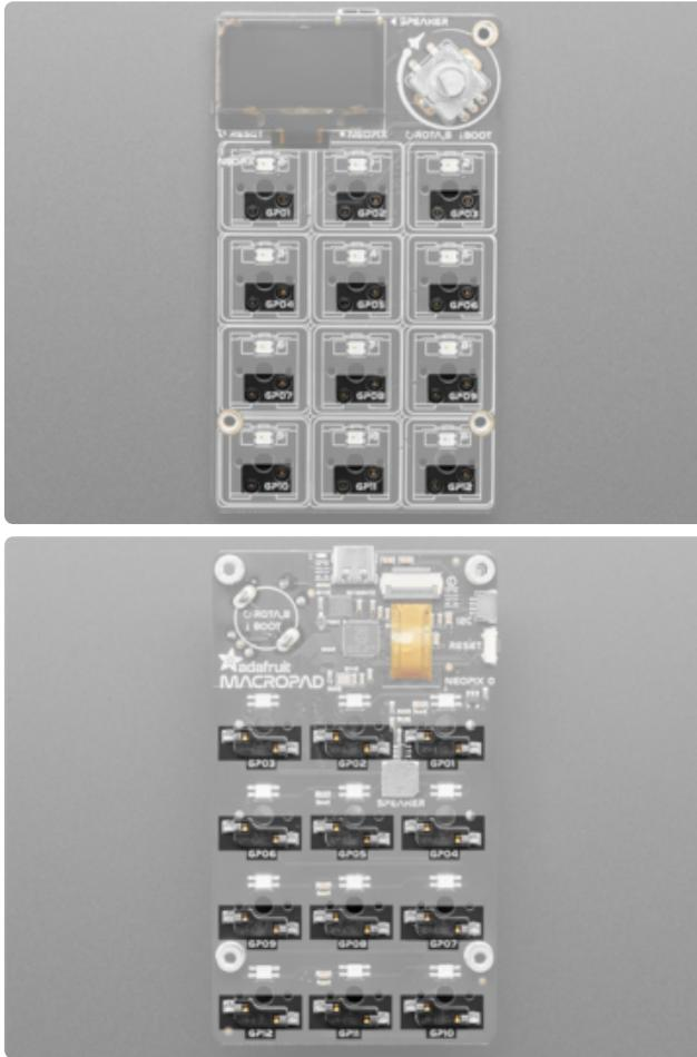
On the MacroPad, laid out in a 3x4 grid, are the Cherry-MX compatible key switch sockets. They are mounted on the back of the board so the socket points through to the front. The key switch sockets are individually tied to GPIO pins (i.e. not matrix-wired).
