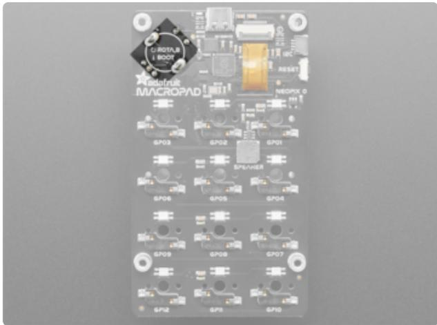
The rotary encoder is available in CircuitPython at `board.ROTA` or `board.ENCODER_A` and `board.ROTB` or `board.ENCODER_B`. It is available in Arduino as `PIN_ROTA` and `PIN_ROTB`.
