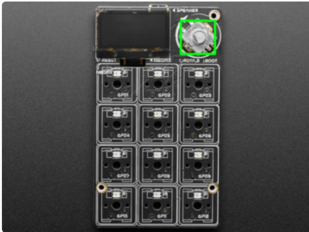
The button (highlighted in green) is located in the rotary encoder - to use the button, simply press down on the rotary encoder.
