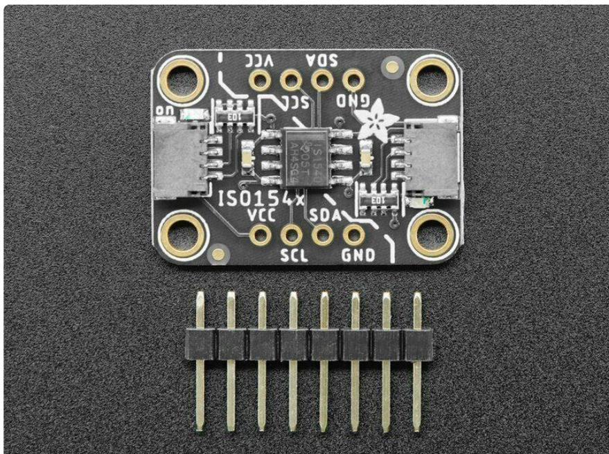
Whatever it is, you can use the Adafruit ISO1540 Bidirectional I2C Isolator to add full electrical isolation between two sides of an I2C bus. The chip we use, the TI ISO1540 is fully bi-directional, supports up to 1 MHz clock rates, supports clock-stretching,
