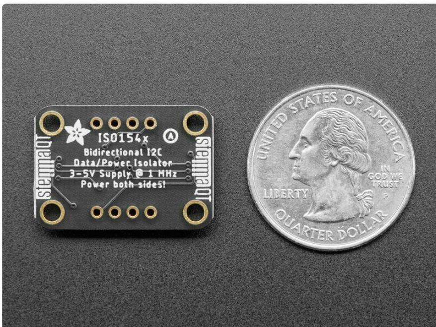
To get you going fast, we spun up a custom made PCB in the [STEMMA QT form factor](#) (), making it easy to interface with. The [STEMMA QT connectors](#) () on either side are compatible with the [SparkFun Qwiic](#) () I2C connectors. This allows you to make solderless connections between your development board and the ISO1540 or to chain it with a wide range of other sensors and accessories using a [compatible cable](#) (). [QT Cable is not included, but we have a variety in the shop](#) ().
