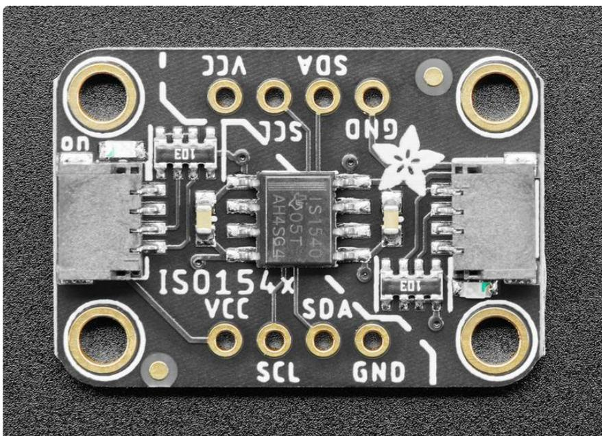
There are TWO SETS of power and data lines that are ELECTRICALLY ISOLATED!
