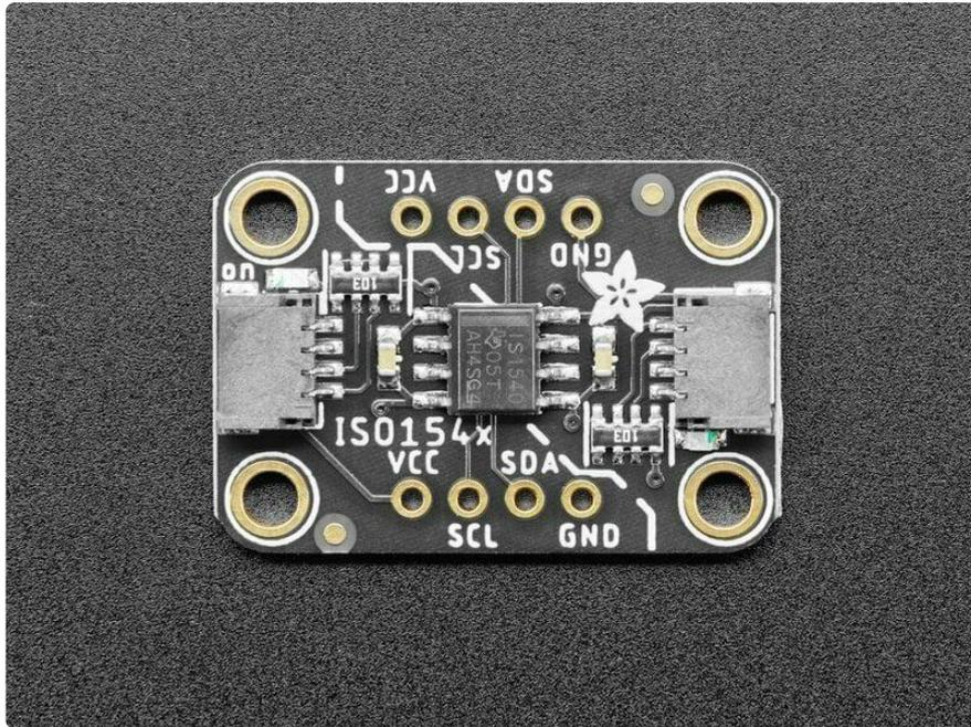
Sometimes you'll find yourself with an I2C bus controller on one side, and an I2C bus device on the other and [you gotta keep em \(electrically\) separated](#) (). Maybe because one is Earth-grounded, maybe because you've got some funky power monitoring setup, maybe you want to reduce noise.
