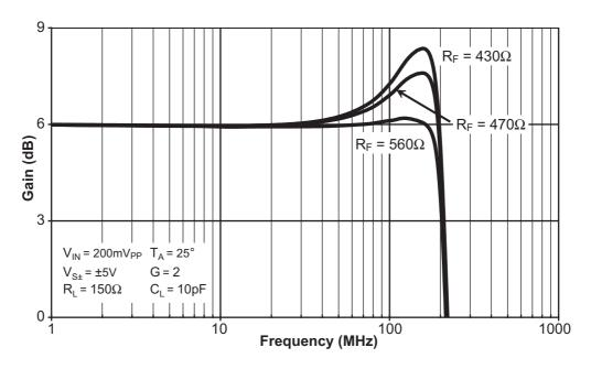
Figure 3 Gain of 2 small signal bandwidth
