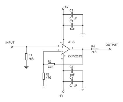
Figure 1 Typical video signal application circuit, gain = 2 (overall gain = 1 for 75 $\Omega$  load
