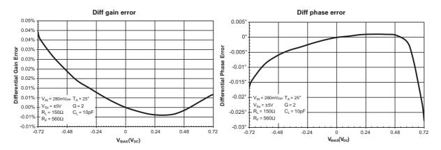
Figures 6 and 7 NTSC/PAL differential gain and phase errors at a gain of 2
