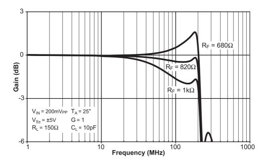
Figure 2 Unity gain small signal bandwidth
