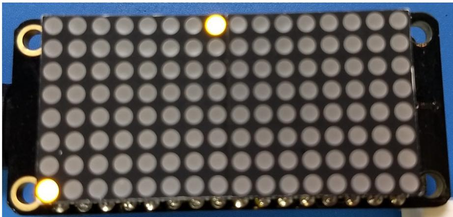
You can also make the entire display blink at 3 different rates using the `blink_rate` property, which has a value 0 to 3:
