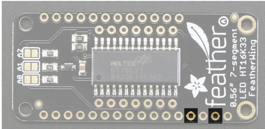
The LED matrix uses only the **3V** and **GND** pins for power and logic. Current draw depends on how many LEDs are lit but you can approximate it as about 40mA for most uses. Check the PCB file/schematic to verify which pin is ground!
