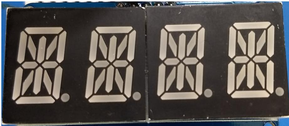
To access the individual digits, it's the same as with the 7-segment display. However, the 14-segment display can take any alphanumeric character. For example:
