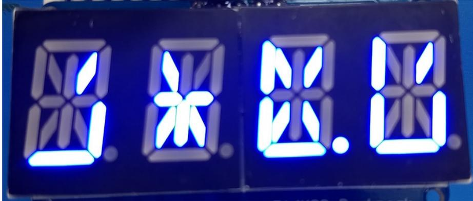
You might notice the display turns on to a 'jumbled' collection of random LEDs. Don't worry! The display isn't broken, right now the module that controls it doesn't clear the display state on startup so you might see noise from random memory values.
