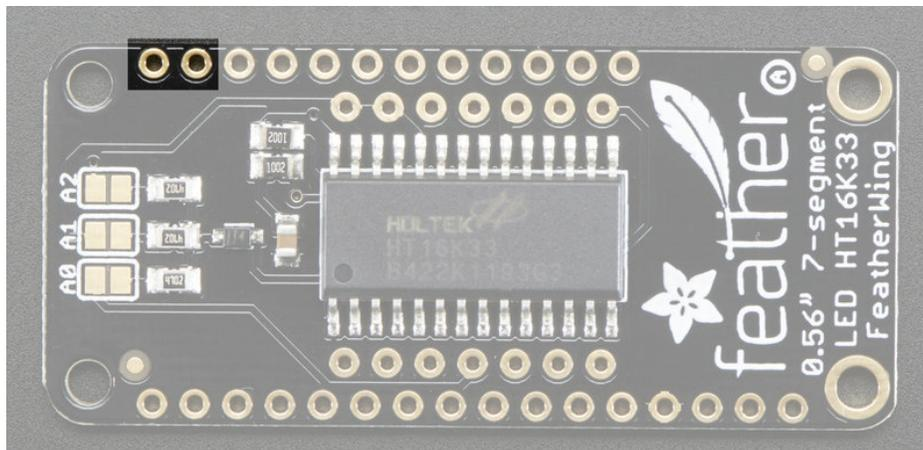
All LED control is done over I2C using the HT16K33 interface library. This means SDA and SCL must be connected, see above for those pins.
