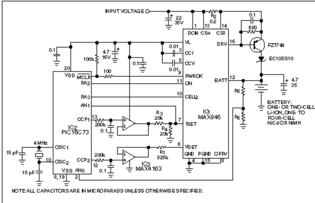
Figure 1. A simple chemistry-independent battery charger combines a microcontroller, IC<sub>1</sub>, with a battery-charging controller, IC<sub>2</sub>, that employs linear regulation.
